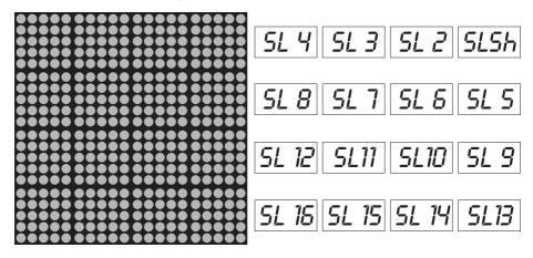
To set one device as master firstly, press MENU button to Choose and confirm (master mode), then press MENU button to Choose and confirm (show mode). Choose and confirm (16pcs using effect), then the second device press MENU button to (master/slave mode), choose and confirm (slave2 mode), the third device choose and confirm (slave2), then set one by one to Choose and confirm (slave2). After 10 seconds or press MENU long time to return to main menu.
