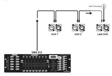
**A word on termination**: DMX is a resilient communication protocol, however errors still occasionally occur. Termination reduces signal errors, and therefore best practices include use of a terminator in all circumstances. If you are experiencing problems with erratic fixture behavior, especially over long signal cable runs, a terminator may help improve performance.
