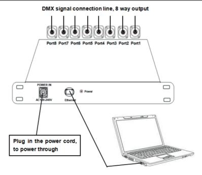
Connect your PC to the DMX control unit using a Cat-5 cable (or USB, depending on control software characteristics - consult with the software seller).
