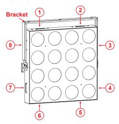
In this way, each module can be easily fixed to another by simply turning the 4 hooks with a hex key.
